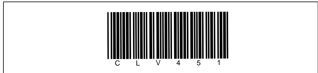
Fig. 6-2: Bar code patter for CLV 451 (Code 39; module width 0.5 mm; Print ratio 2:1)
