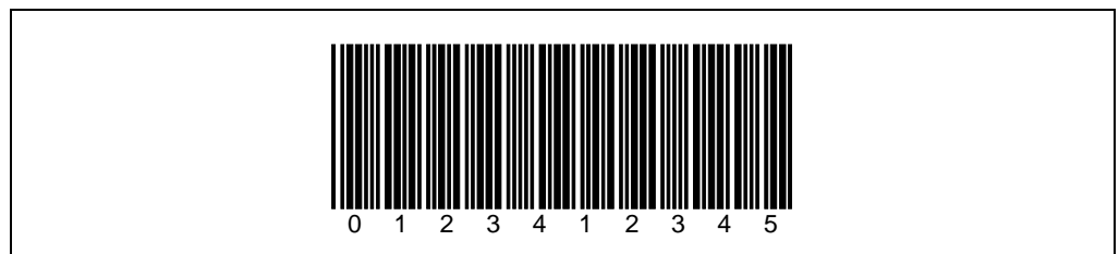
Fig. 6-1: Bar code patter for CLV 450 (Code 39; module width 0.35 mm; Print ratio 2:1)
